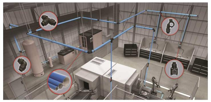
With a modular design and easy-to-assemble components, EPL piping system empowers you to easily plan and adapt your distribution piping network to the needs of your production environment.
